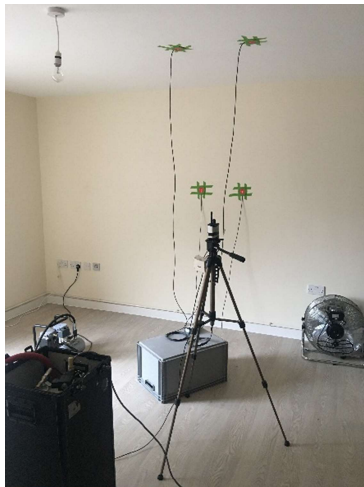
Figure 6: Heat flux plates in place on party surfaces in the top floor flat at FT262 and FT263.
