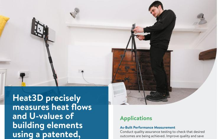
It can be used to detect heat flow rates, thermal bridging, poorly performing structures, as well as assessing existing levels of insulation. Heat3D is designed to work on iPhones and iPads and uses a portable thermal camera to obtain results in a matter of hours as opposed to days or weeks using traditional techniques. The rapid nature of the measurement enables quantified U-values
