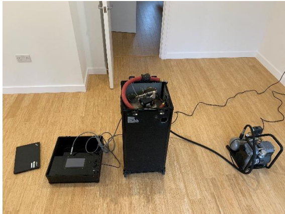
Complete 40L Pulse set-up used in this configuration for all test cases
