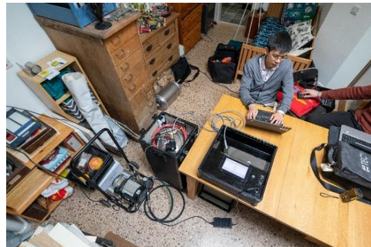
Pulse and blower door fan testing in a small 94m 3 art studio
