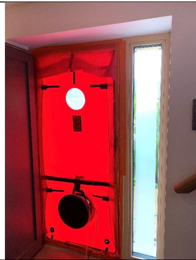
Blower door fan setup in a doorway and taped from inside
