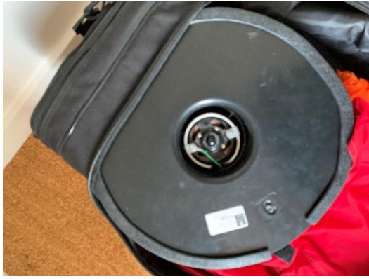
Very low flow min fan required for the fan tests, with large restrictor plate fitted
