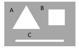
The panel supplied by BTS is pre-tested in a suitably calibrated lab so that the 4Pa flow rates of each hole are precisely known. The Pulse customer then executes a test with different combinations of holes covered. This gives a multi-point check (8 possibilities) which means the testing can happen in any room with background leakage present, providing that a baseline test is taken before the known opening test panels are opened up.
