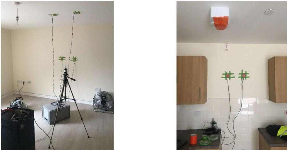
Figure 6: Heat flux plates in place on party surfaces in the top floor flat at FT262 and FT263.
