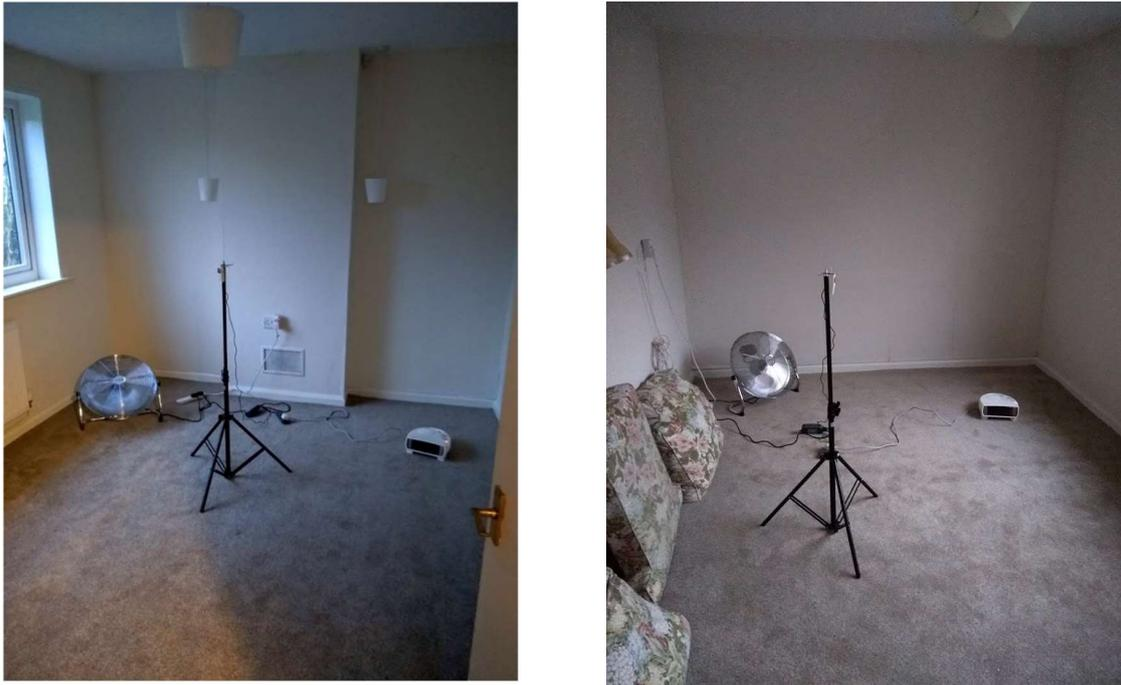
Figure 5: Example installations of thermostatically controlled heaters and air mixing fans.
