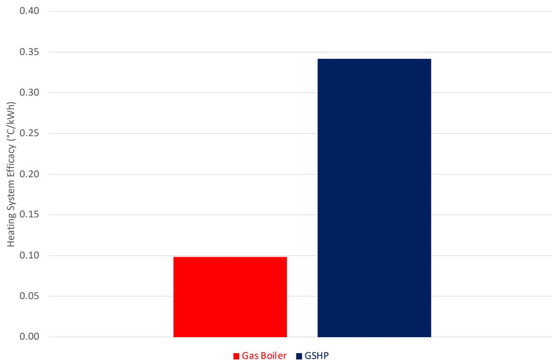
Figure 11: Comparison Between System Efficacy (°C/kWh) of Gas Boiler and GSHP Systems
