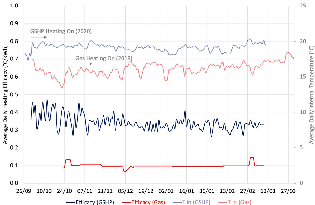
Figure 9: Comparison Between Internal Temperature and System Efficacy for Gas and GSHP Systems
