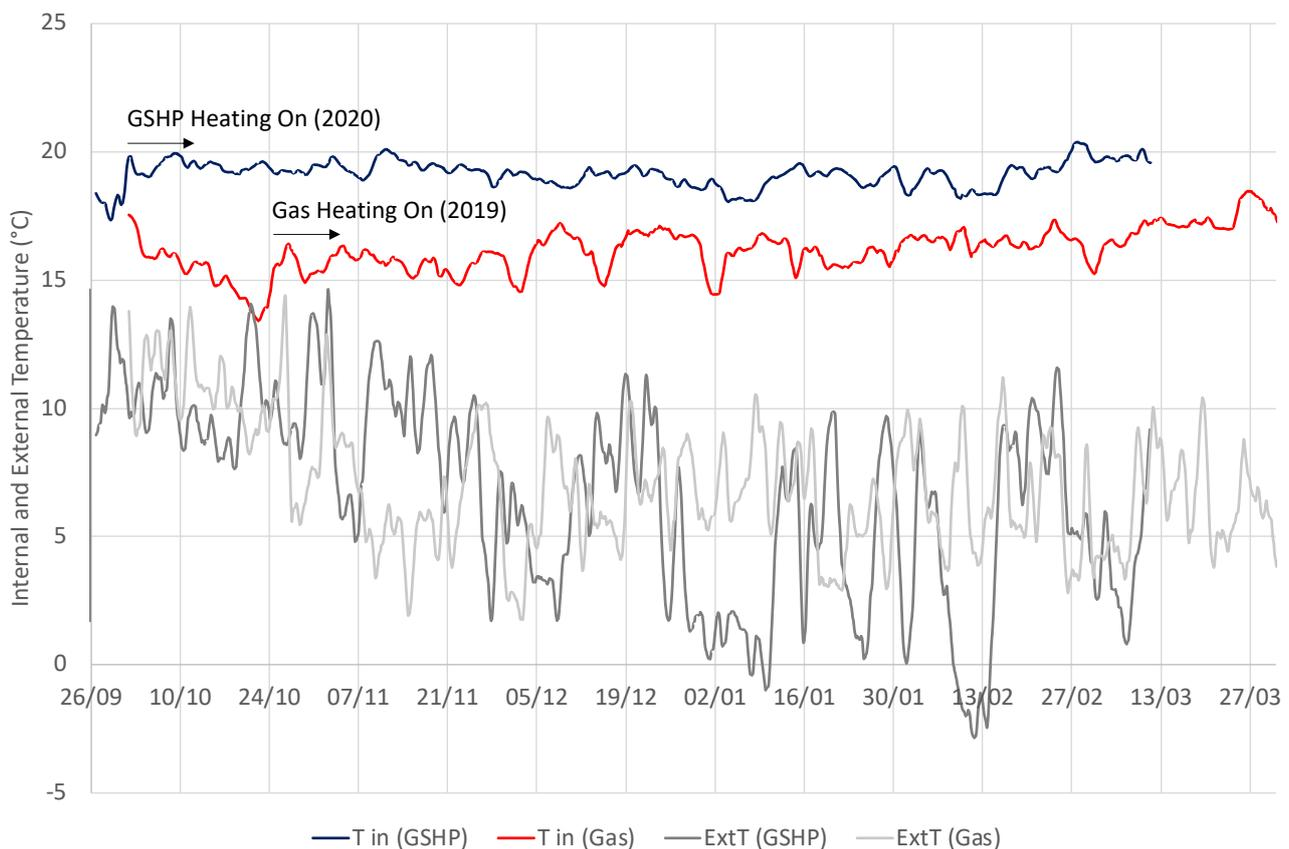
Figure 7: Comparison between Internal and External Temperature During Winter Periods with Gas and GSHP system
