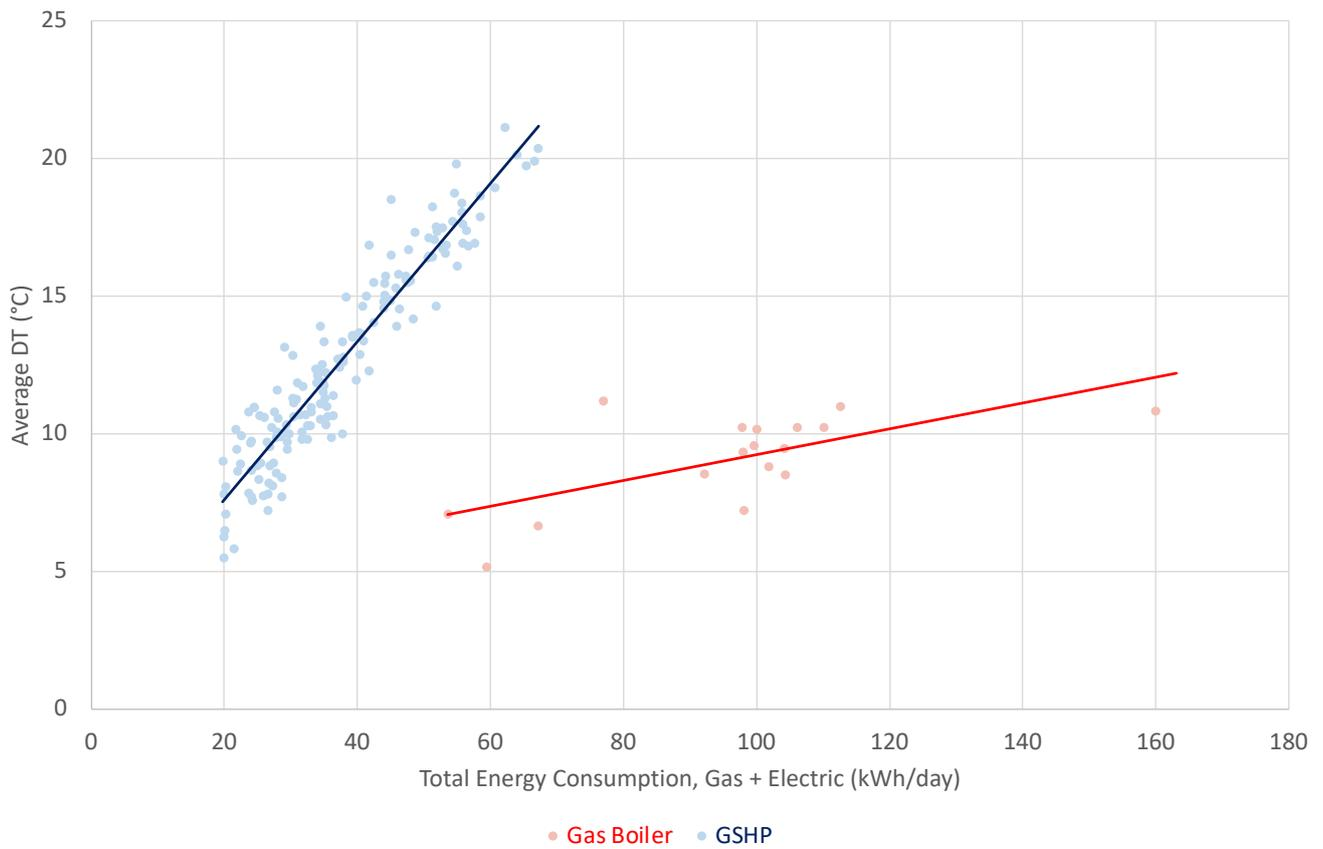
Figure 10: Correlation Between  $\Delta T$  and Total Energy Consumption for Gas and GSHP Systems
