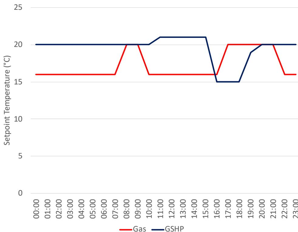
Figure 8: Temperature Setpoints for Gas Boiler (2019) and GSHP (2020) Systems
