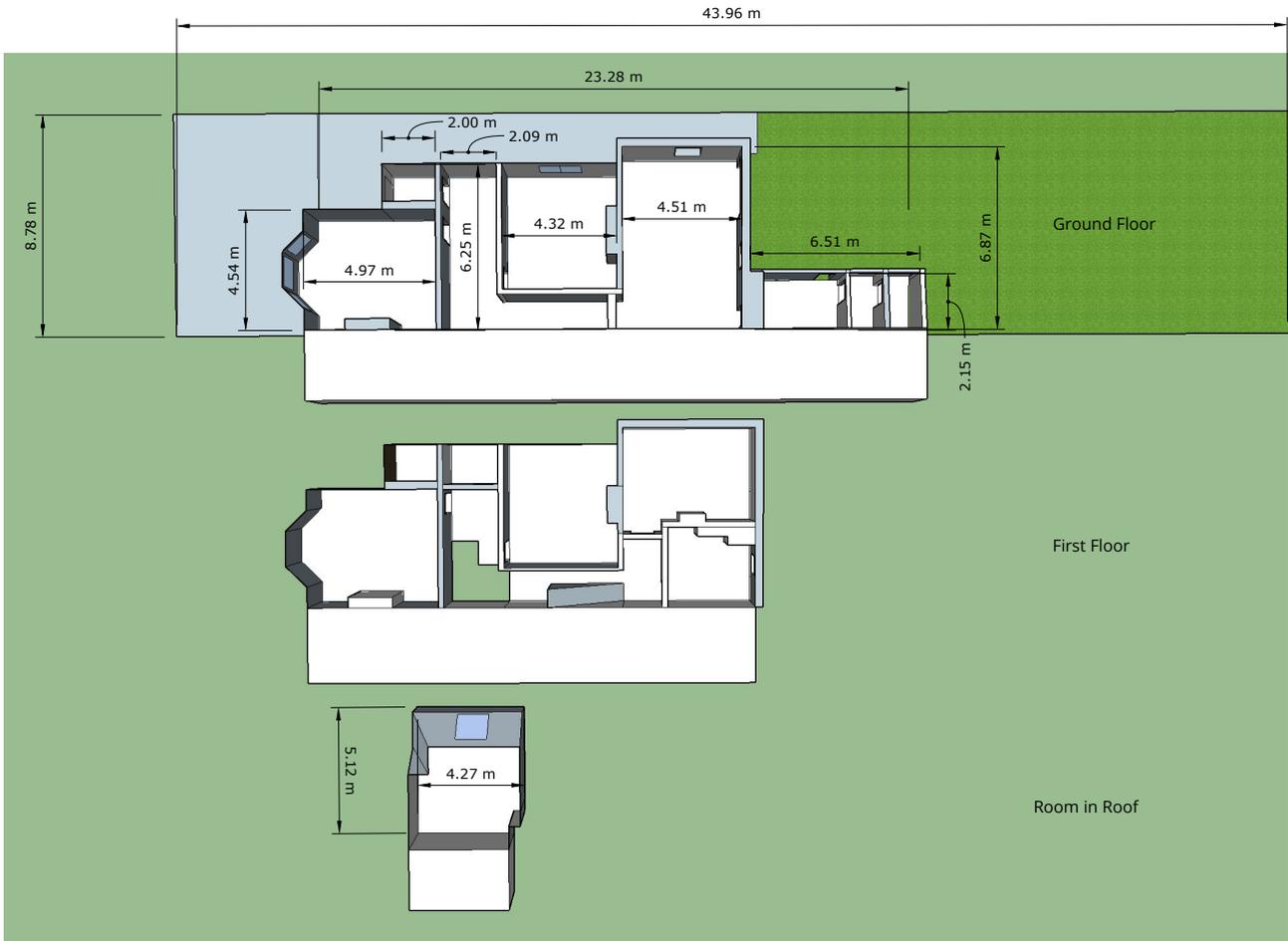
Figure 2: As-Built Floor Plan
