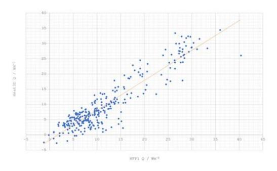
**Figure 1:** Field trial results showing a comparison of measured Heat Flow (Q) from industry standard Heat Flux Plate (HFP1) and the developed Heat3D system for a range of building structures
