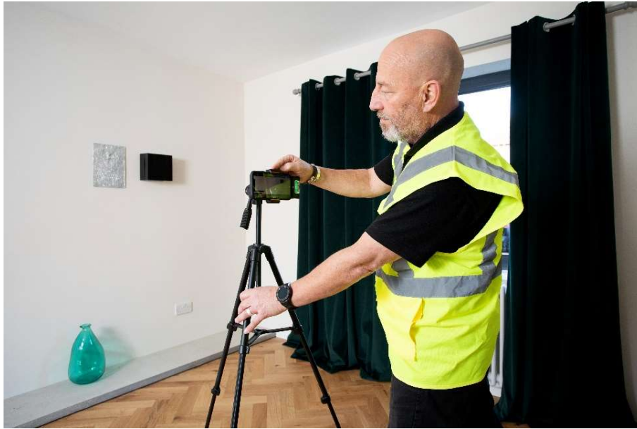
Figure 2: An example of a Heat3D time lapse-survey being set up, with device and tripod in the foreground and air and reflected temperature targets in the background.
